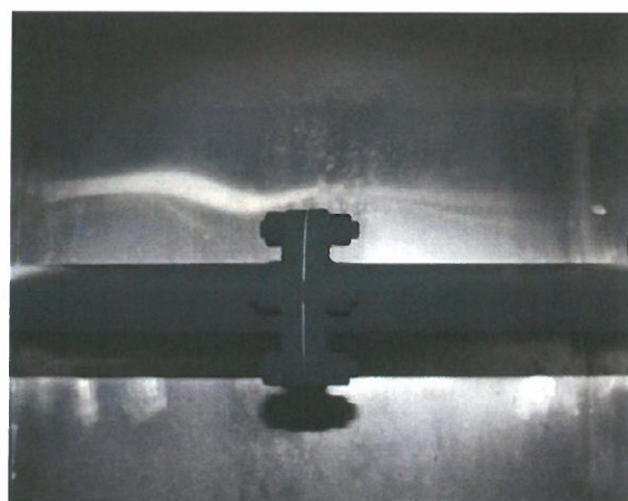
[Photo 4] Hydrostatic tightness test
