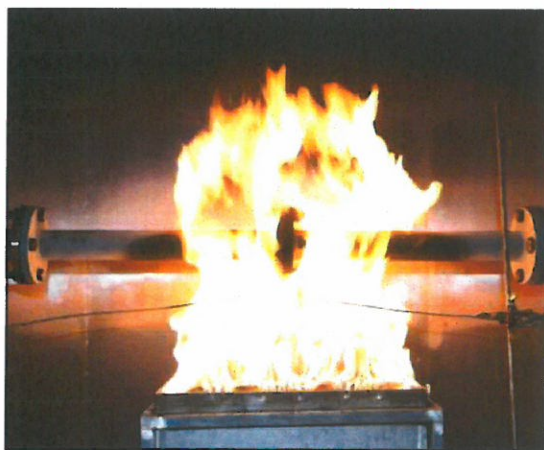
[Photo 3] Fire endurance test
