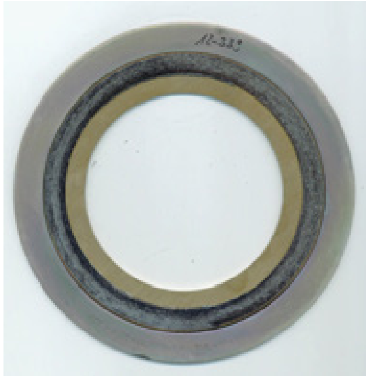
Shell cycle test (T) according MESC SPE 85/300 - 3.3.5
