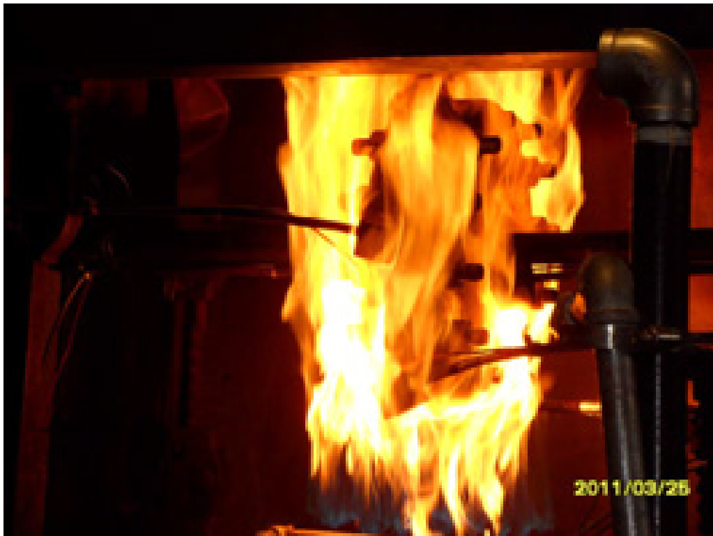
Gasket Fire Test
