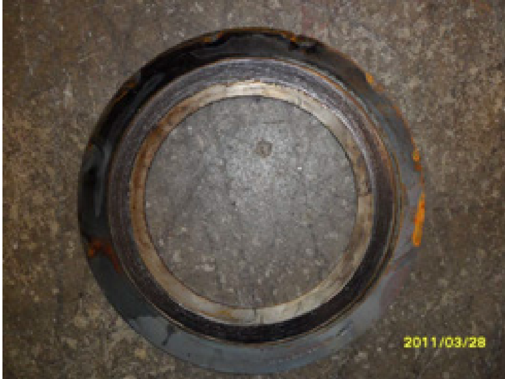
Gasket After Test
