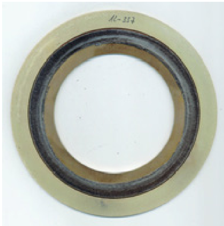
Shell leakage test (T) according MESC SPE 85/300 - 3.3.2
