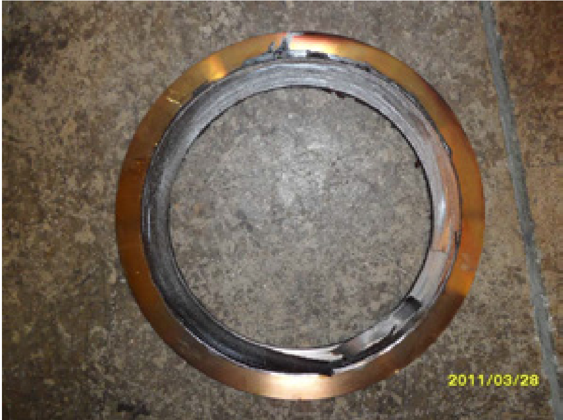
Gasket After Test
